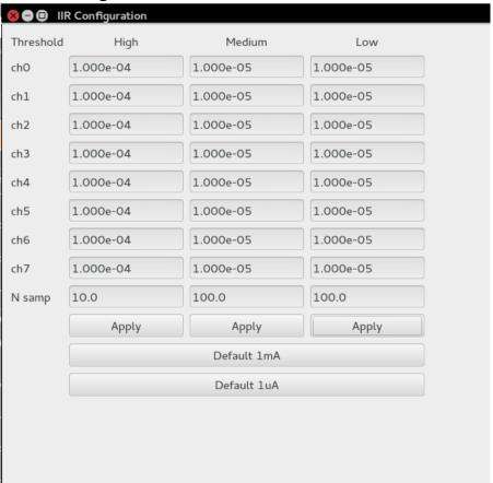
From this menu it is possible to configure all the thresholds and the number of samples on which the moving average is performed.
