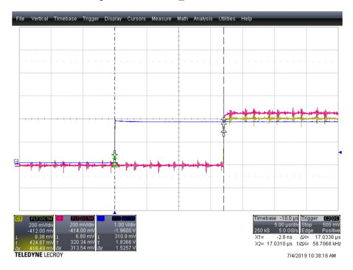
This is the delay from an input signal (blue curve) to the MPS generation. We configured the AMC-PICO8-MPS in order to generate the MPS signal just with  $\bf ONE$  sample over threshold. The latency is 17 us = 1 us (sampling) + 16 us (FMC-PICO-1M4 analog filter).
