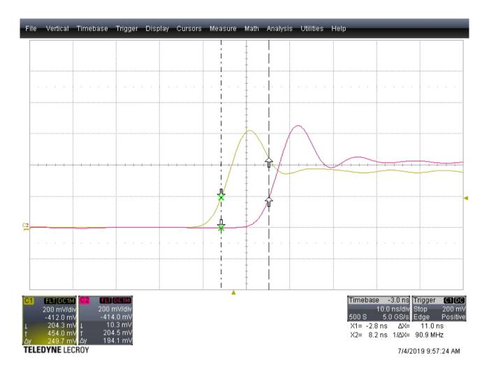
This is the latency between one board (AMC-PICO8-MPS) and a fake TPCTRL (in this case a DAMC-FMC25). As you can see, the backplane connectivity is very fast, 11 ns to send the signal from the AMC-PICO8 to the TPCTRL.
