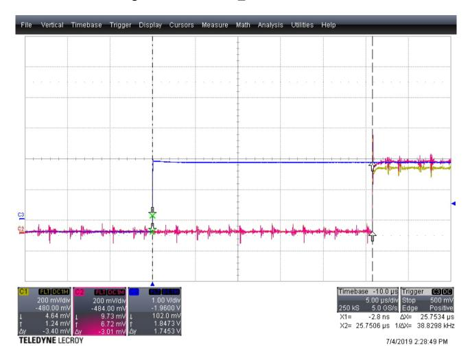
This is the delay from an input signal (blue curve) to the MPS generation. We configured the AMC-PICO8-MPS in order to generate the MPS signal  $N_SAMP = 10$  samples over threshold. The latency is around 26 us = 10 us (sampling 10 values) + 16 us (FMC-PICO-1M4 analog filter).
