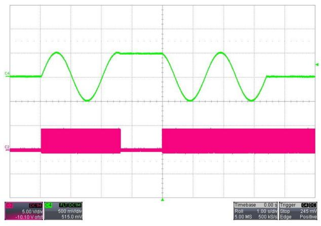
• Example #3: WAVE:TRIGGER:GATE with TRIGGER:HIGH option
