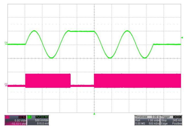
• Example #3: WAVE:TRIGGER:GATE with TRIGGER:HIGH option
