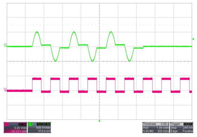
• Example #4: WAVE:TRIGGER:GATERESET with TRIGGER:HIGH option
