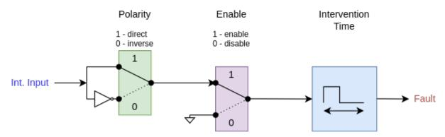
The interlock intervention time specifies how much time the interlock condition should be valid in order to trip the interlock fault. It is also possible to set the intervention time to  $0 \rightarrow$  in this case the fault trips immediately, when an interlock condition is detected.
