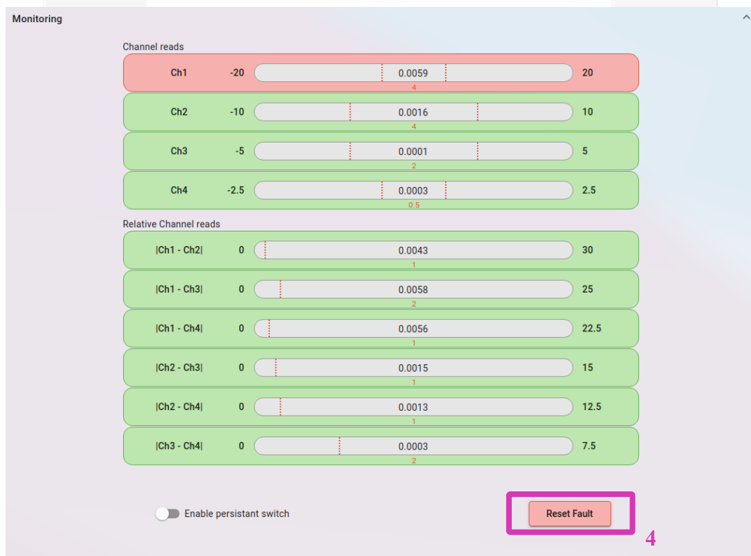
Figure 5: Monitoring menu in fault condition.
