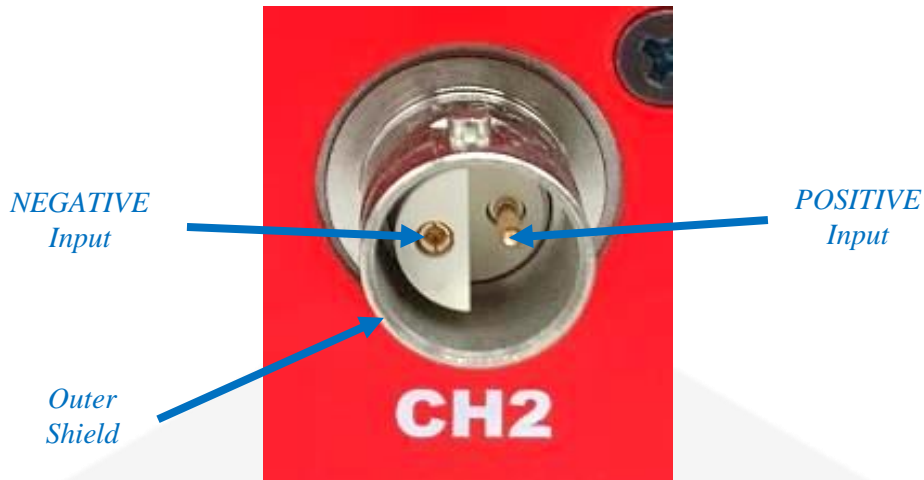
Figure 16: Pinout for the TWIN BNC connector
