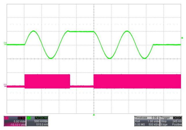
• Example #3: WAVE:TRIGGER:GATE with TRIGGER:HIGH option
