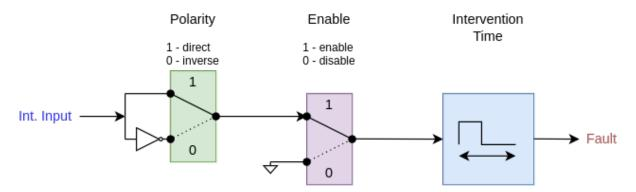
The interlock intervention time specifies how much time the interlock condition should be valid in order to trip the interlock fault. It is also possible to set the intervention time to  $0 \rightarrow$  in this case the fault trips immediately, when an interlock condition is detected.
