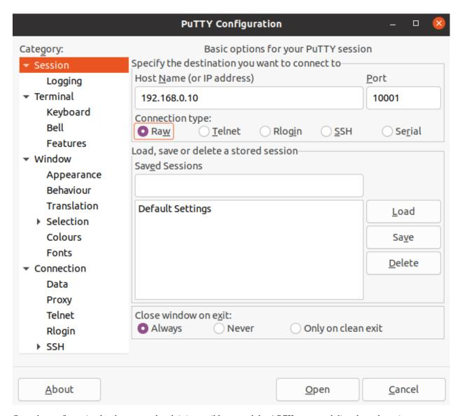
Once the configuration has been completed, it is possible to send the ASCII command directly to the unit:
