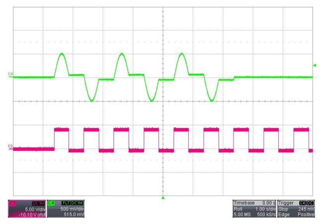
• Example #4: WAVE:TRIGGER:GATERESET with TRIGGER:HIGH option
